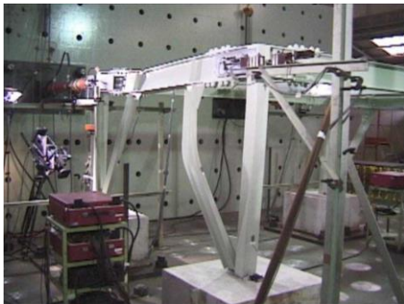
Photograph-5 The compression braces were completely buckled by the static load experiment
