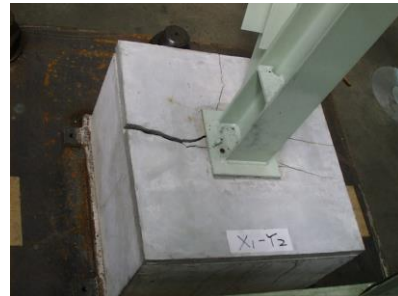
Photograph-4 Pedestal was broken by ductile fracture (Type-0)
