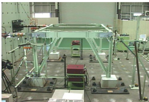
Photograph-2 Static load experiment without reinforcement model (Type-0)
