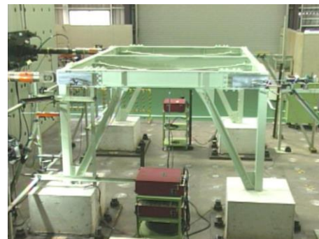
Photograph-3 Static load experiment with reinforcement model (Type-3)
